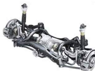
Newly developed five-link rear suspension shown with available quattro® all-wheel drive
