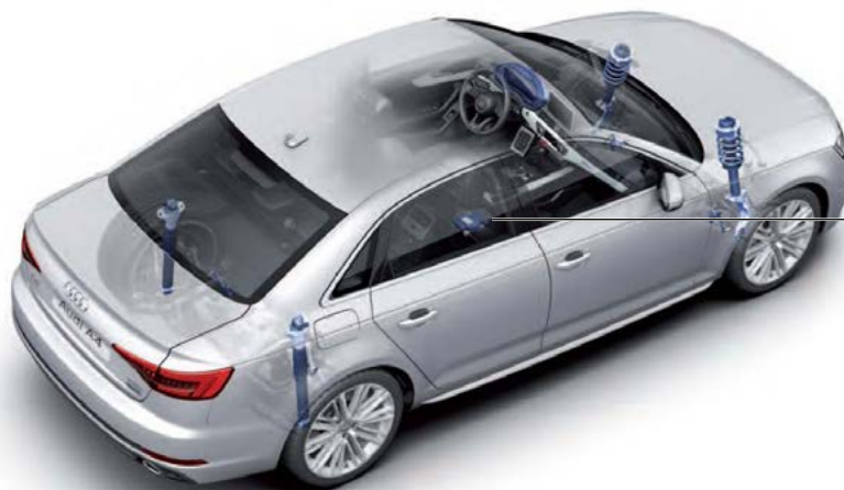
New adaptive damping suspension control unit
